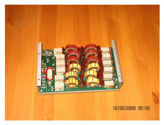
Desolder RL 13 and replace with a new one
